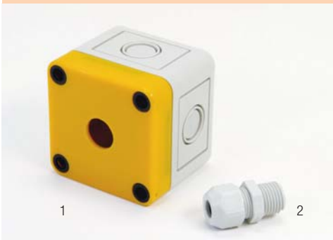
Emergency-stop switch enclosure with 16mm mounting hole, 65mm (w) x 65mm (h) x 57mm (d) and cable gland M16
