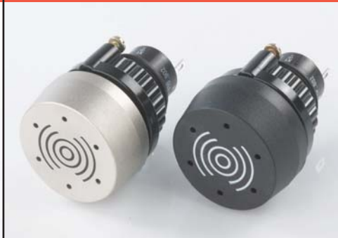
Buzzer, plastic bezel, raised, 22.5mm mounting, 24VDC, IP65, 95dB ± 8 at a distance of 0.1m
