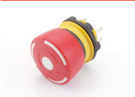
Emergency-stop non illuminated, plug-in terminals, twist release, 32mm diameter for 22.5mm mounting, foolproof to EN 60947-5-5
